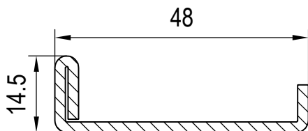
|FI| 229063 s=2.0mm 4.3/0.2cm4 Reinforcements
